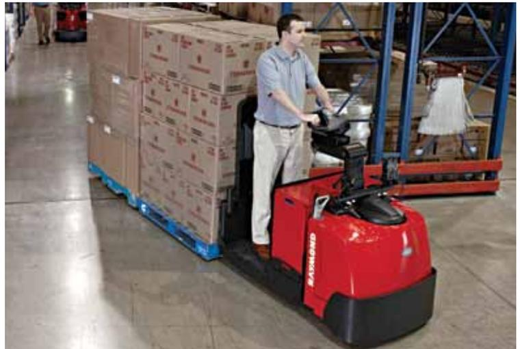
On the Model 8510 center rider and Model 8610 tow tractor, PowerSteer automatically slows the truck when cornering, to maintain operator control.
