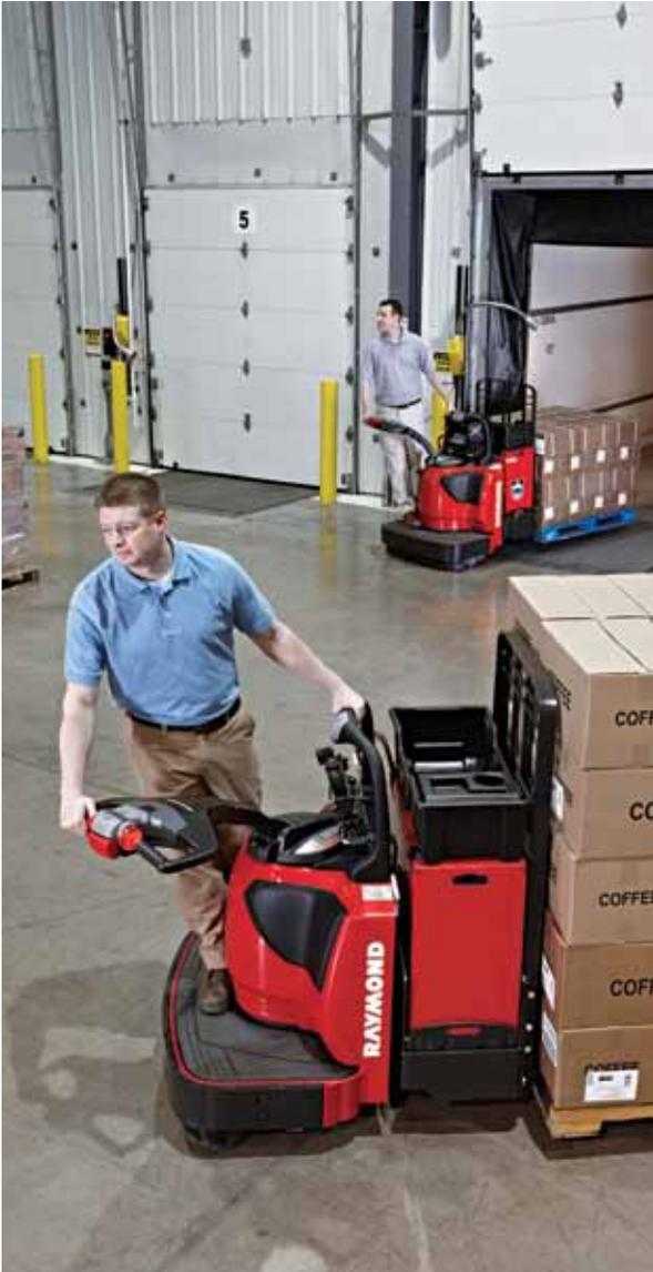
On the Model 8410 pallet truck, speed-sensitive steering provides steer assistance when it's needed most – at slower speeds. And operators appreciate the smooth, controlled operation at all speeds.
