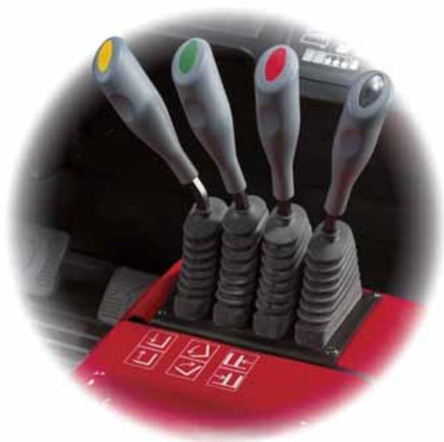
Convenient color-coded levers control lift, lower, tilt and side-shift.
