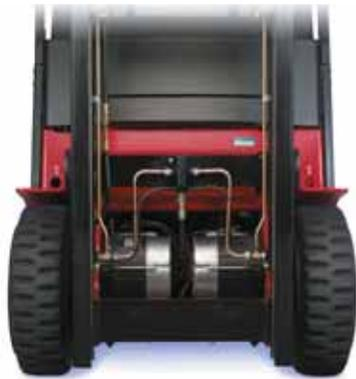
The 4700 Series trucks lead their class in maneuverability. Dual AC drive motors on the C30, C40 and C50HM models provide a tighter turning radius.
